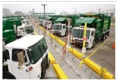
collection vehicles at its 50 fueling bays. More trucks are expected to be added within the year! The vehicles fuel overnight and run for 10-12 hours on 50 gallons of fuel. CNG fuel runs more quietly than diesel and prevents air pollution. Because natural gas is domestically available and runs more cleanly than oil, these types of facilities are encouraged in the Will County Energy & Conservation Plan.
